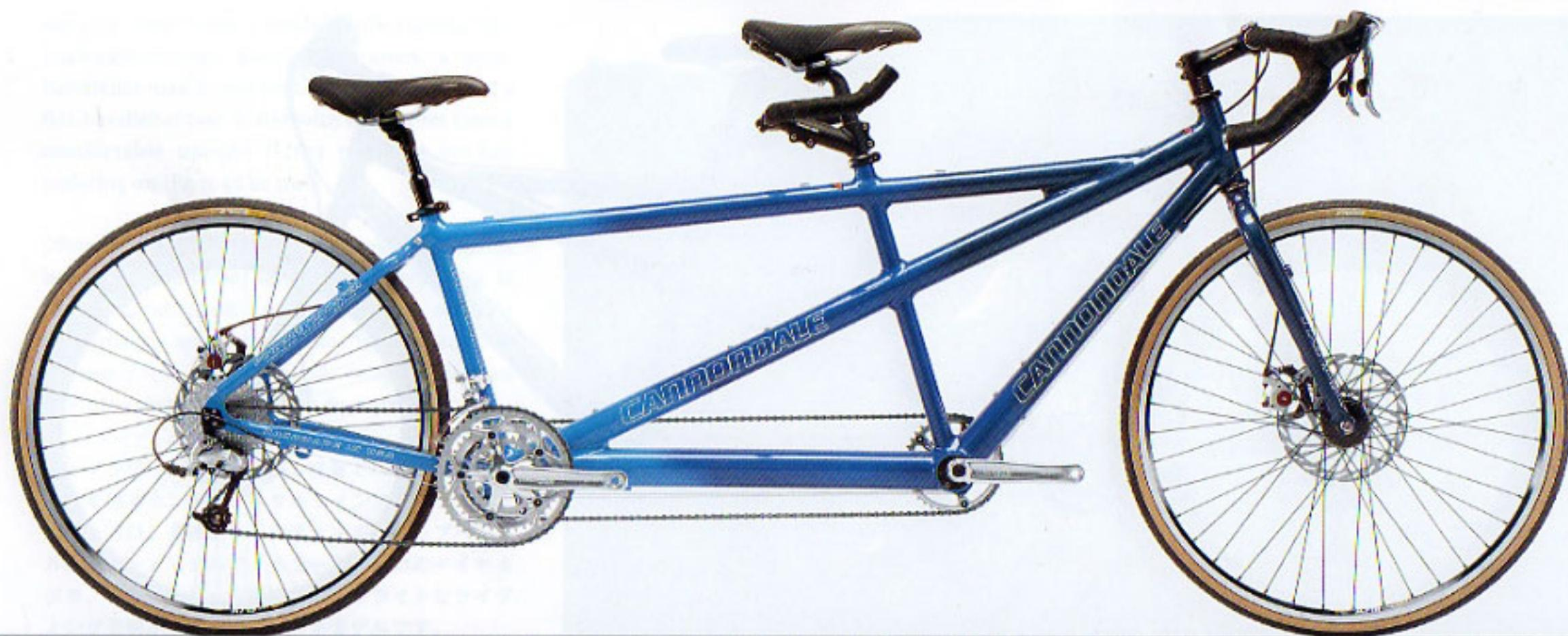
• Road Tandem frame • Fatty R Tandem fork • Mavic A719 rims with DT Tandem Disc hubs and Champion spokes • Shimano Ultegra 9-speed shifters with XT rear derailleur • TruVativ Elita crankset with ISIS bottom brackets • Avid BB7 disc brakes • 1X Suspension seatpost • MS, LS, XS, XM, JL • Midnight Blue to Patriot Blue to Blazer Blue (gloss) (BLU); Platinum (gloss) (PLT)
