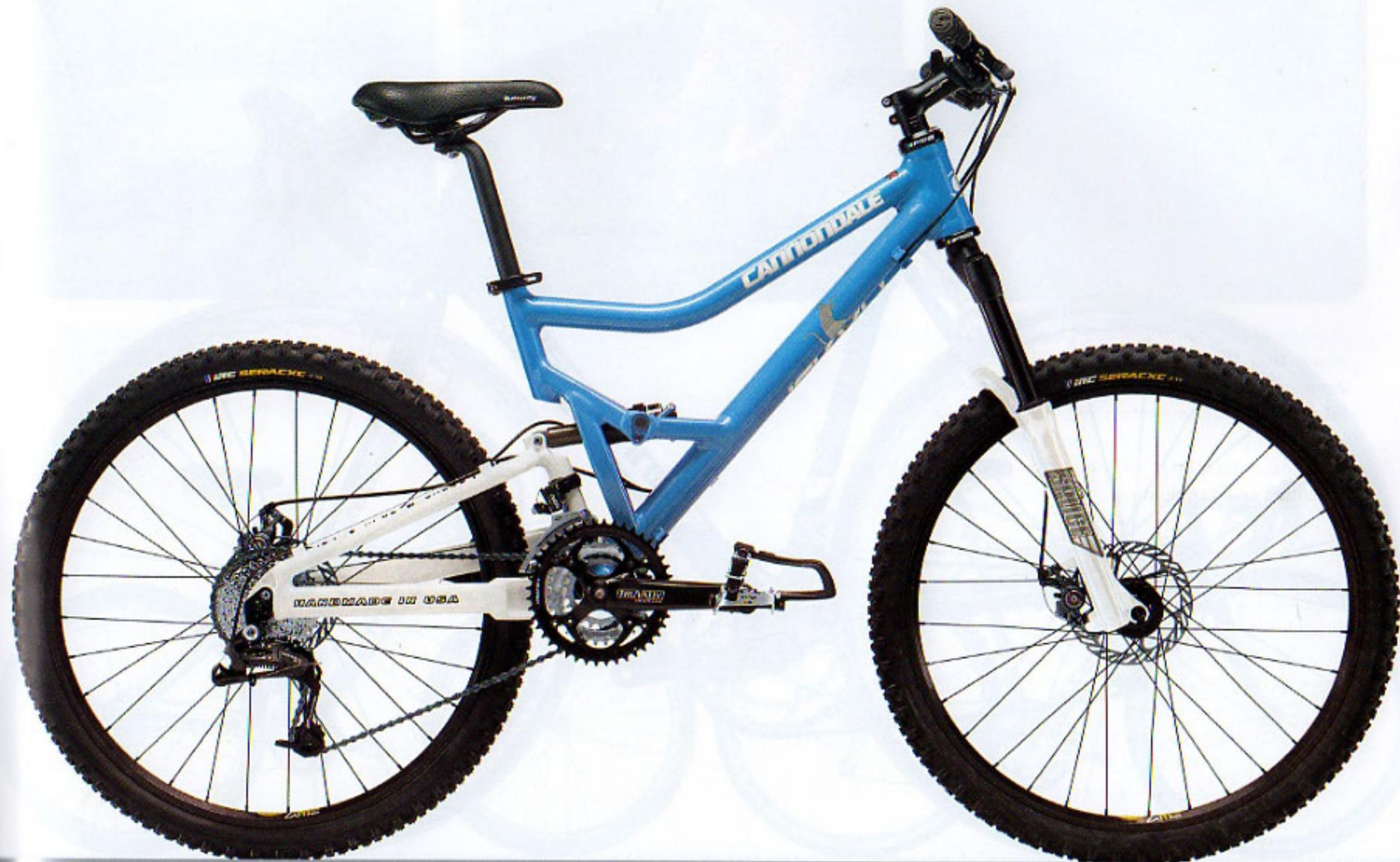
• Jekyll Féminine frame • 135 mm of rear wheel travel • Adjustable Bottom Bracket height • Manitou Splice Super Diva 100-130 fork w/RTWD • Fox Float RL ProPedal Air rear shock • Avid BB5 disc brakes • P, S, M • Blazer Blue w/Lightning White swingarm (gloss) (BLU); Lightning White w/Sterling Silver Hyperhighlight (gloss) (WHT)
