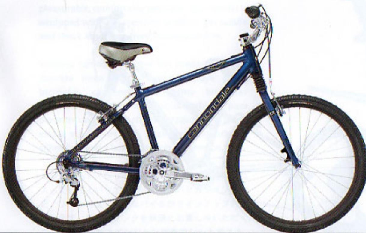
• Comfort HS frame • HeadShok Fatty 50 All-Conditions fork • Mach1 210 rims with DT Stainless spokes • IRC Advantage Pro tires • SRAM MRX Pro shifters • Shimano Deore rear derailleur • Adjustable rise stem • 1-X Suspension seatpost • Super Cush Gel saddle with Springs • S, M, L, X, J • Jet Black w/Patriot Blue HyperHighlight (gloss) (BLK); Platinum (gloss) (PLT)
