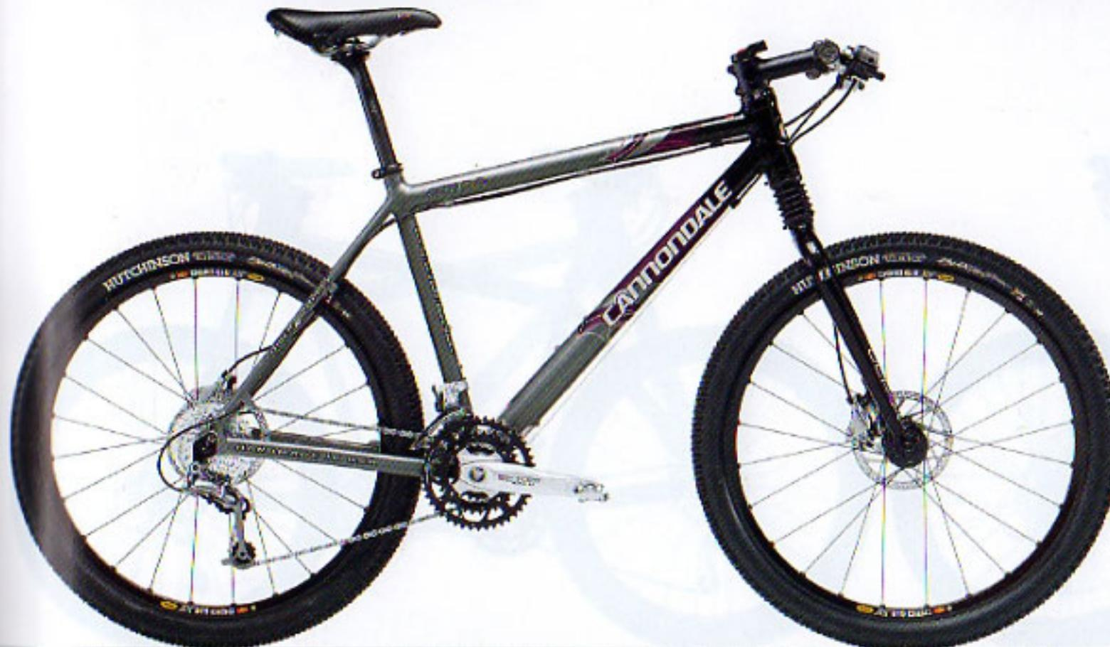
• Optimo frame • Compliant hourglass seatstays • HeadShok Super Fatty Ultra DLR fork • Shimano XT crank
