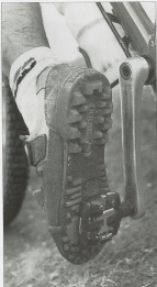
Click and go: Shimano's SPD system stays in use to work about flipping the clip (left). The "clip" step of the spring-loaded mechanism and it locks in the recessed slot in the bottom of your shoe.
