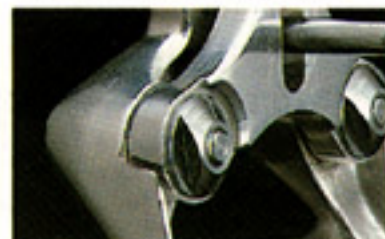
Sealed Mechanism preventing mud, water and unwanted objects from entering for smooth braking at all times.
