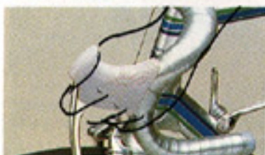
Undulations which spread palm pressure power evenly
