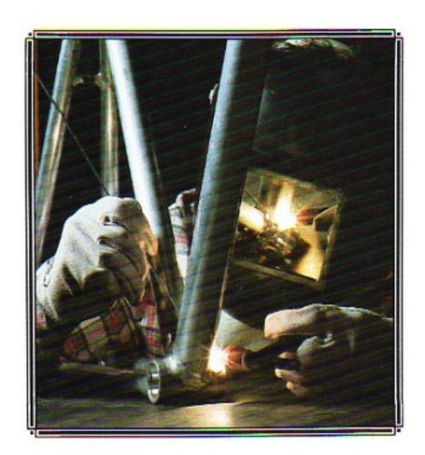
Our tubing is precisely mitered to within strict tolerances, then it is securely and accurately fixtured for TIG welding by our trained welders. TIG (Tungston Inert Gas) welding is the strongest way to join aluminum. It is a sophisticated process using an electrical arc shielded by inert gas that makes clean, strong aluminum welds. The welds on a Cannondale frame are the work of skilled professional craftsmen.
